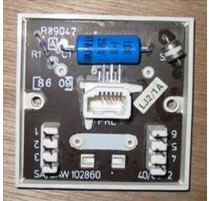
Remove any wires attached to terminals 4 and 6 and 1 and 3 (the top and bottom on both sides, only the middle connections 2 and 5 should have anything attached).
