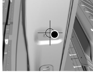
G 后门锁扣安装孔 \Phi 9 Rear door swith mounting hole
