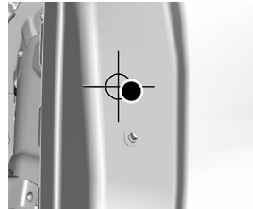
G 后门锁扣安装孔 \Phi 9 Rear door swith mounting hole
